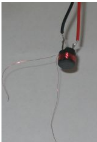
10mH choke with 150 turns for the secondary
