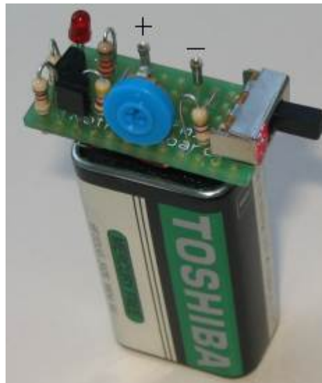
The regulator connected to a 9v battery
